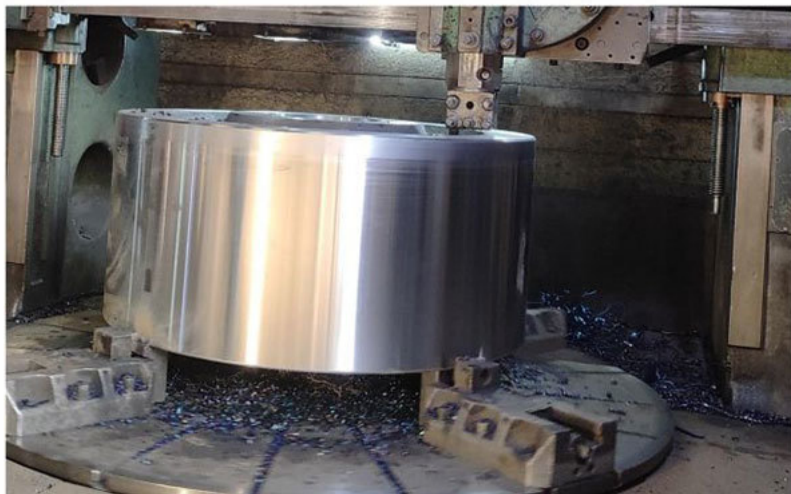
Chemical plant trunnion roller
